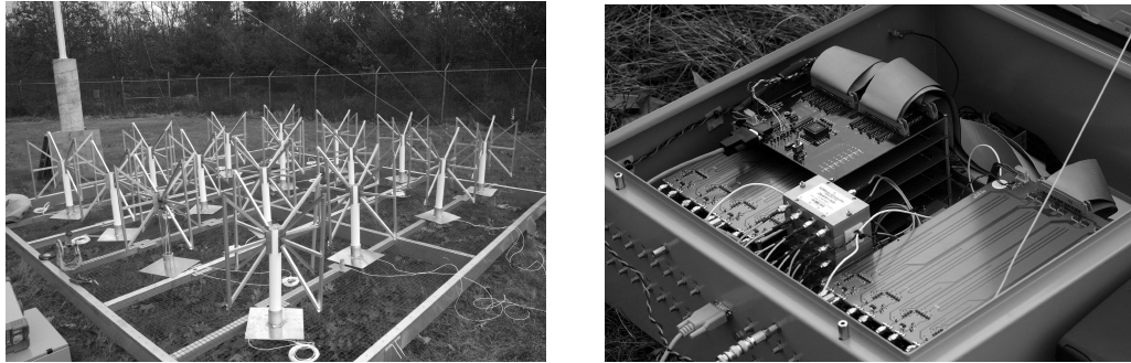
Figure 3. A 16-dipole antenna tile and beamformer used in tests at Haystack Observatory.
