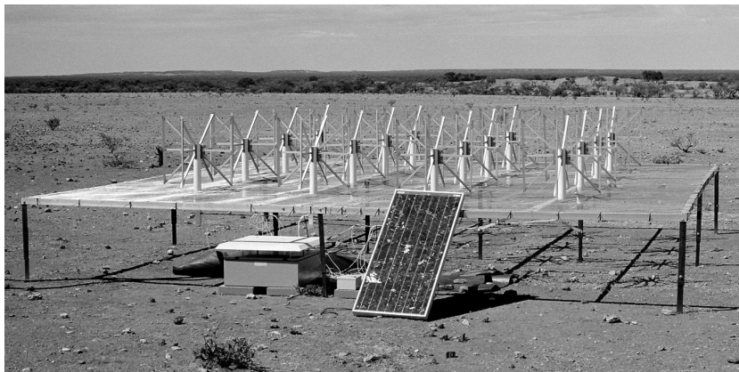
Figure 5. The first completed antenna station with beamformer box and battery-backed solar power supply.
