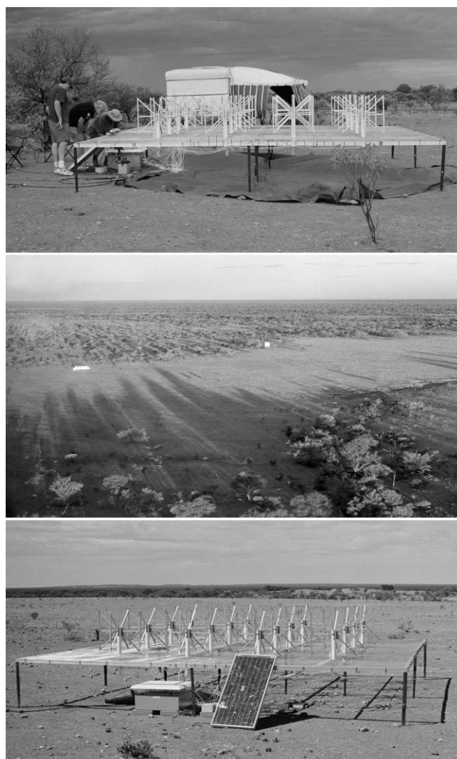
FIG. 1.—Photographs of the first MWA LFD prototype antenna tile being tested on site in Mileura, WA, Australia. The antenna consists of 16 crossed dipoles in a 4 \times 4 m grid and is elevated approximately 0.8 m above the ground. Top : Antenna tile being assembled near the caravan used for housing the computers and receiver electronics. Middle : Aerial view after the antenna tile was moved to its final location, approximately 150 m northwest of the caravan. Bottom : Completed antenna tile in position. The solar panel is visible leaning against the tile, and the beamformer box and heat shield are under the tile. Two additional antenna tiles were subsequently installed at the site. [See the electronic edition of the Journal for a color version of this figure.]
